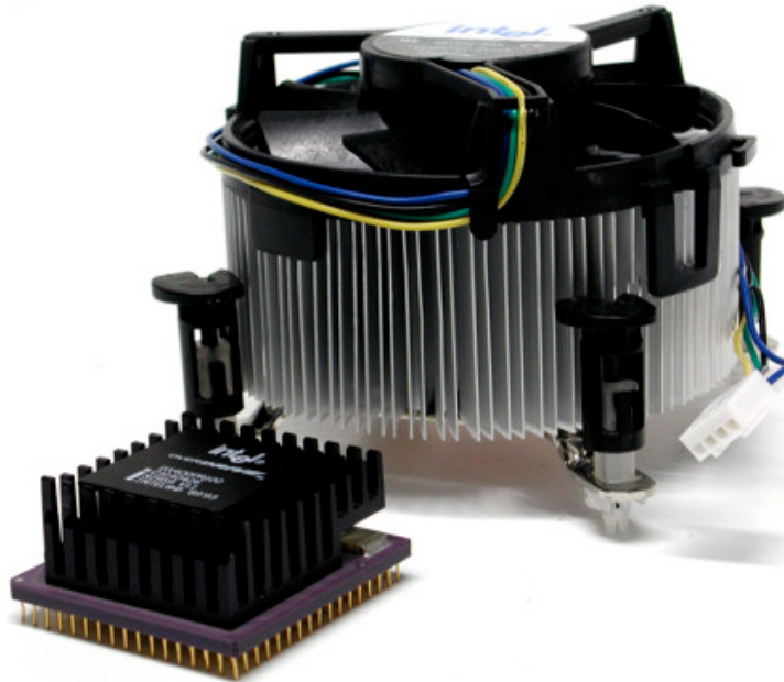
Figure 1.6: Pentium Overdrive “chip and heat sink” from 1993 (bottom left); standard Pentium 4 “heat sink only” from 2005 (top right).
