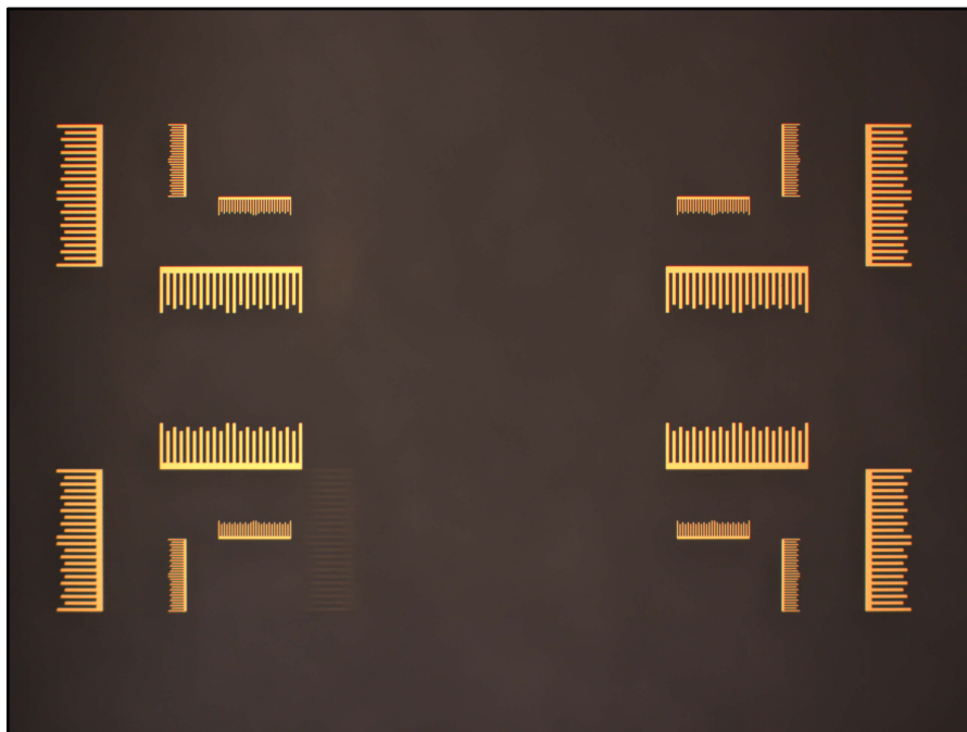
Figure 94. Optical image of fabricated Vernier scales used for alignment measurement characterization. The resolution of these Vernier scales is 1 μm.
